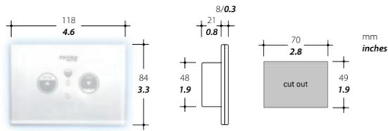
Multiframe SFT control panel [Compatible with all commercial bezels: B-Ticino, Vimar, Gewiss, ABB, AVE]:
