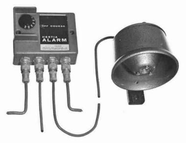
The "off-course" alarm system is installed in conjunction with the HESTIA course indicator. It emits a penetrating tone when the ship's head departs by more than a certain pre-determined angle from the set course. It is intended primarily for use in the following applications:—
