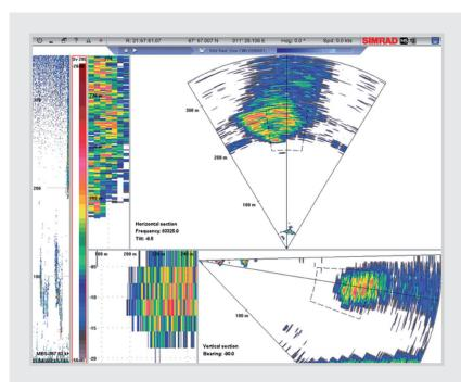
This screenshot shows a school of herring. Even though the MS70 detects and records data from all 500 beams, only two sectors can be shown in a traditional 2D view. One is a horizontal slice, while the other is a vertical slice through the matrix. In addition to that, you can have a zoon view and an echogram from the single beam shared by the two sectors.
