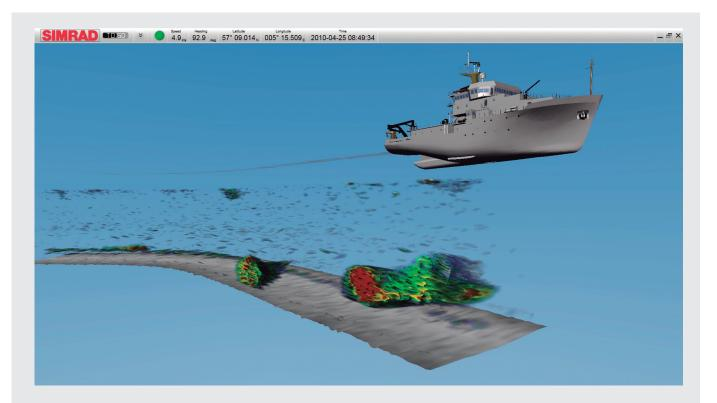
The Simrad TD50 Multibeam 3D Visualisation Software is shown presenting sand eels on sand bottom. The raw data is taken from the Simrad ME70 Scientific multibeam echo sounder on M/S Simrad Echo.
