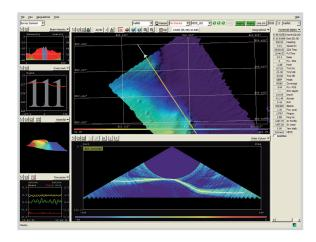
Kongsberg's own Seafloor Identification System (SIS) is also included in the delivery, adding an extensive set of graphical displays for data quality control, as well as system calibration, data cleaning, gridding, and visualization.
