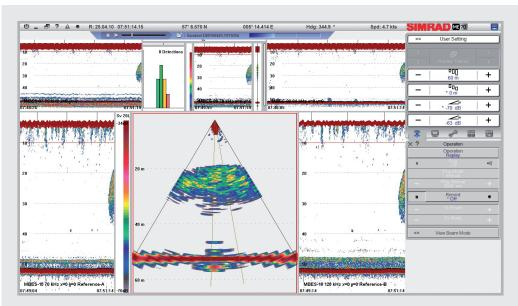
Here we have a screenshot from the ME70 acquisition software. On the centre of the image we see the combined swath of beams athwartship. The software is flexible: it not only shows the individual beams of your choice, but you can also see split beam information, such as size, from each beam.
