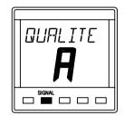
Press **SIGNAL** key to complete the change. The LCD now shows French text.
