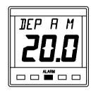
Press **ALARM** key, the alarm is displayed.
