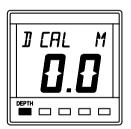
Press **DEPTH** key to display depth datum **D CAL M**.
