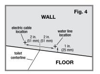
These locations are for the water and electrical supply line holes in through-the-wall installations.
