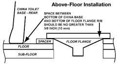
STEP 8: Cut out the 4-3/4-inch (120 mm) diameter discharge flange hole. Drill the two 3/16-inch (5 mm) holes mounting bracket fastener holes. Where required (floor or wall), drill the 1-inch (25 mm) diameter water line hole and 1 3/4-inch (44 mm) electrical wiring hole.
